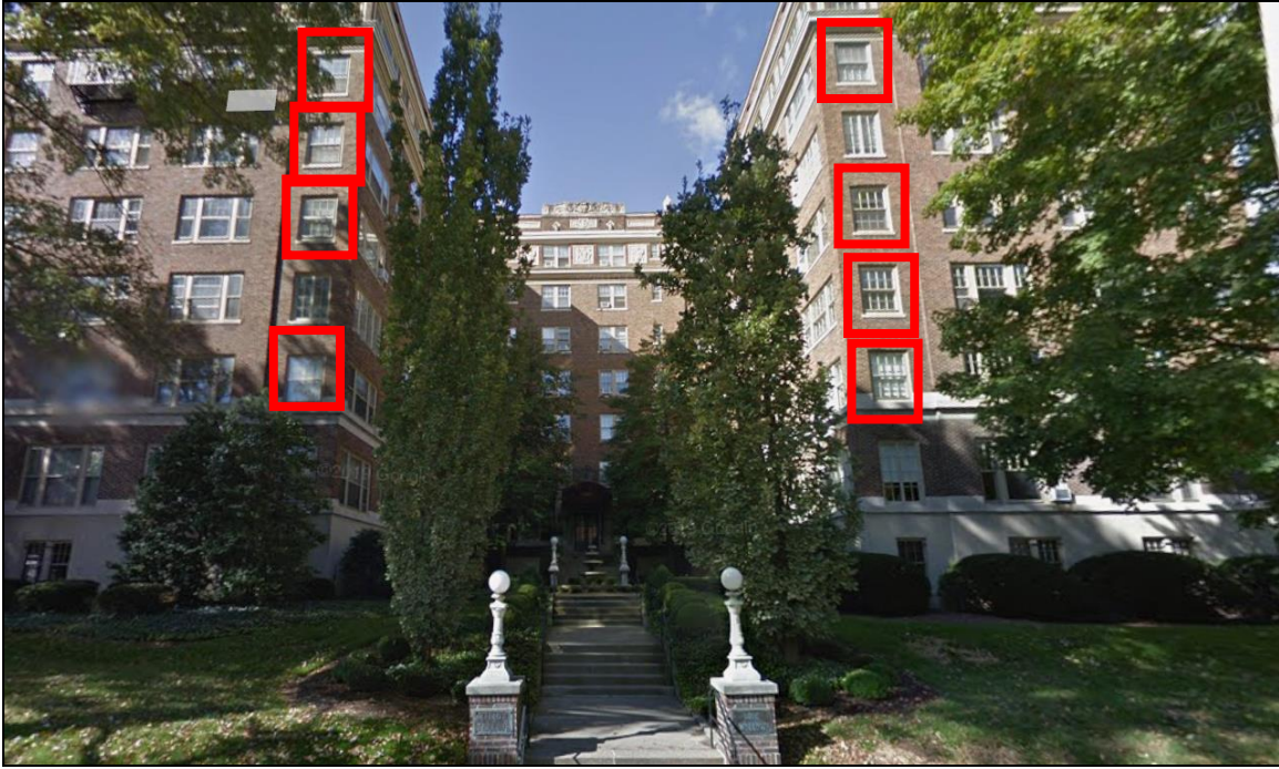
Figure 2 – Google Street View, Oct 2018, of 1412 Willow Ave. (red squares indicates a 16-lite casement window previously replaced with a 16-lite double-hung window).
