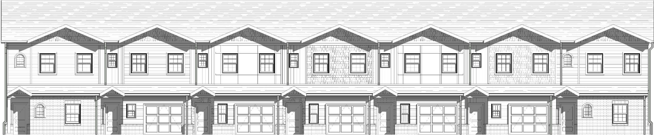
1 20' UNITS - TYPICAL FRONT ELEVATION 3/16" = 1'-0"
