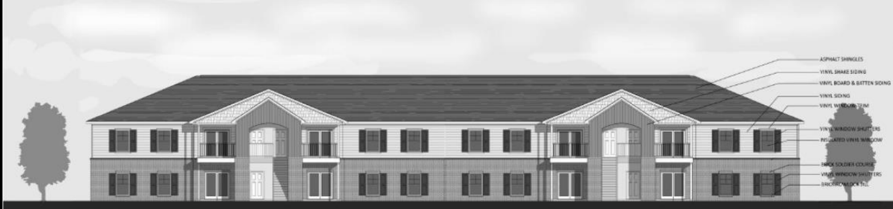
1 A1.1 2 BED REGULAR BUILDING ELEVATION Scale: 1/4" = 1'-0"
